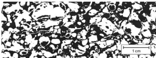
Figure 1 Phenolic foam prepared for quantitative image analysis, showing the contrast between cell voids and solid phase.
